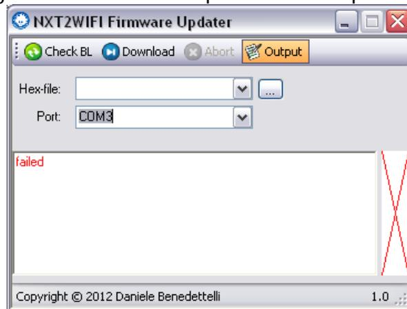
5. Select the COM port of your device from the Port drop down menu. To check if the device is correctly connected and communicating with the Firmware Updater program, press the reset button on the device and click the Check BL button at once (actually within 1 second since the reset). You should see the PIC type and the bootloader version in the log window.
