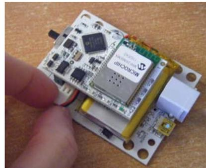
3. The new battery might be not completely charged. Connect the device to your computer using a miniUSB cable: the red "Charge" led is on until the battery is fully charged. Turn the device on using the power switch: the green light on the Wi-Fi module will turn on. **The first time you turn the device on, it automatically connects using the DEFAULT connection profile to an adhoc network called "NXT2WIFI". After activation, you have to connect it manually (keep reading).**
